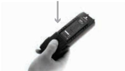
After short calculations, the LED indicators will light up to display the current battery charge level. ADII's battery level indicator has 5 LEDs that show how much power is remaining. See the table below for details:
