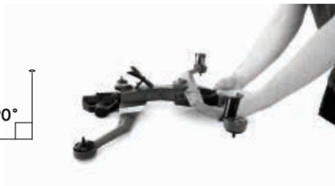
23. A message: **"CALIBRATING Hold steady"** will appear, do not move the drone while this message is visible.
