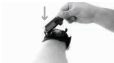
Then press down and secure the other side of the strap clamp:
