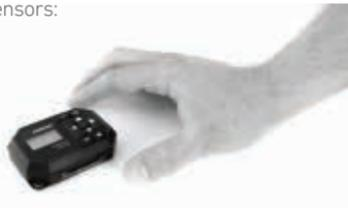
12. Calibration will start after 5 sec., a message stating: “**CALIBRATING don't move**
