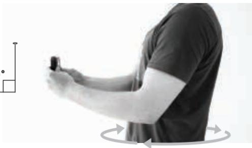
15. Hold AirLeash steady with indicated side UP until you hear a tone and see a message: **"Rotate 360° holding
