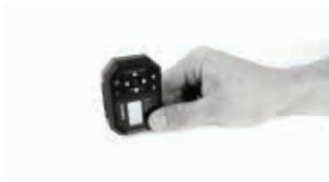
17. Place AirLeash on a level surface steady at a 90° angle (relative to the surface) so the displayed message is readable. A message: **"CALIBRATING Hold steady"** will appear, do not move AirLeash while this message is visible.
