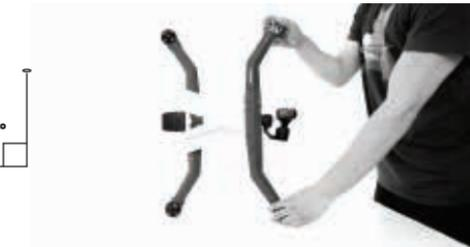
21. A message: **"CALIBRATING Hold steady"** will appear, do not move the drone while this message is visible.
