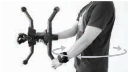
19. When you hear a different tone and see the message: **"Rotate 360°, holding
