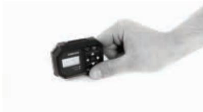
13. Place AirLeash on a level surface and hold it steady at a 90° angle (relative to the surface) so the displayed message is readable. A message: “**CALIBRATING Hold steady**” will appear, do not move AirLeash while this message is visible.
