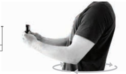
17. Hold AirLeash steady with indicated side UP until you hear a tone and see a message: **"Rotate 360° holding steady"**, rotate ONLY when you see THAT message.
