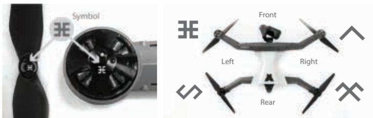
To attach the propellers you have to match the propeller symbol with the same symbol on the motor. Note that front arm motors are facing down, so start with the rear arms and then flip the drone belly-up and attach the front propellers.
