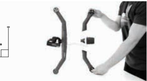
19. A message: “**CALIBRATING Hold steady**” will appear, do not move the drone while this message is visible.
