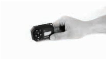
15. Place AirLeash on a level surface steady at a 90° angle (relative to the surface) so the displayed message is readable. A message: “**CALIBRATING Hold steady**” will appear, do not move AirLeash while this message is visible.
