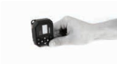
19. Place AirLeash on a level surface and hold it steady at a 90° angle (relative to the surface) so the displayed message is readable. A message: **"CALIBRATING Hold steady"** will appear, do not move AirLeash while this message is visible.
