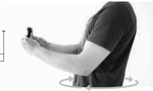
19. Hold AirLeash steady with the indicated side UP until you hear a tone and see the message: **"Rotate 360° holding [AirLeash icon] steady"**, rotate ONLY when you see THAT message.
